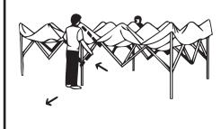
Go to each corner of the frame and engage the auto slider by pushing up with one hand while holding down the top of the leg with the other hand. This should then click into place. Repeat on all other legs.
