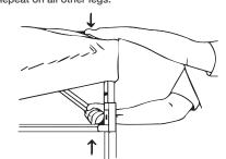
Lift two adjacent outer legs up and pull out the inner legs until they click into your desired height. We recommend extending the legs to the 3rd or 4th hole. You will need to ensure your marquee is secured by using the supplied pegs or ask about our leg weight accessories.
